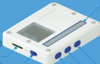
40-Pin GPIO Header
