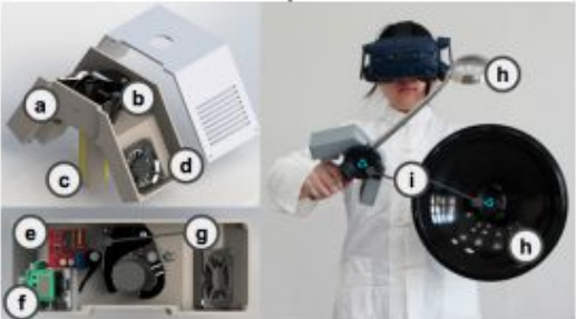
Figure 2: Hardware design: (a) 1/4" Screw, (b) c-clamp, (c) heater, (d) fan, (e) mini L298N, (f) LinkIt 7697 with Robot Shield and battery, (g) vibrator, (h) prop, and (i) Vive tracker.
